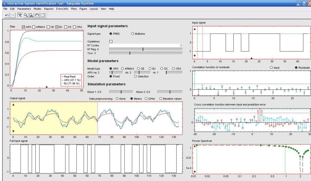
Figure 2.3: ITSIE interactive tool user interface for two cycles of a PRBS input applied to a simulated fifth-order system, with selection of different parameters from the Input signal parameters menu.
