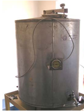
Fig. 5.10 Insulated filling tank
