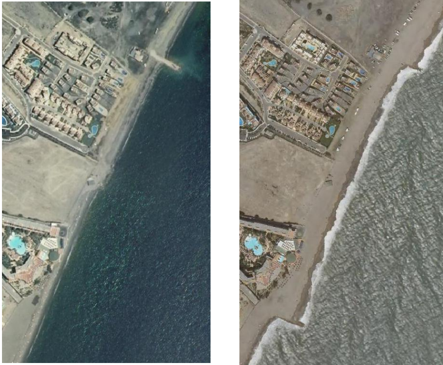
Figure 4.10. Coastal evolution according to the jetties emplacement. In the left, activities regarding the construction (2007, official web map service source) are shown. In the right, first year stages of the construction and the sand nourishment is presented (2008, official web map service source).
