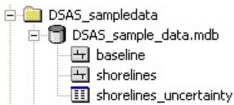
Figure 7. View of the sample data from ArcCatalog. The DSAS_sample_data.mdb geodatabase contains baseline and shoreline feature classes along with an example of an advanced-use shorelines_uncertainty table.
