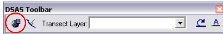
Figure 16. Screenshot showing the DSAS Toolbar application. The circled button launches the Set Default Parameters window.
