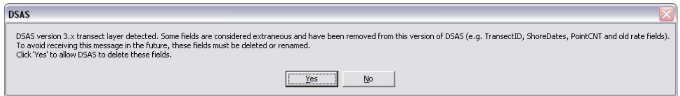
Figure 29. Screenshot of warning message that users may encounter when DSAS recognizes transects from previous versions of DSAS. This message will appear if any of the extraneous fields listed in the message are detected in the transect feature class attribute table.
