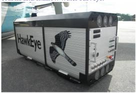
HawkEye simultaneously collects 4000 bathymetric measurements (full waveform) 64000 topographic measurements (up to four returns per shot), which makes the system to the most efficient airborne bathymetric LiDAR survey system available at the world market. With the maximum swath of 330 meters and a typical aircraft speed of 75 meter per second, the system surveys up to 350 square km per day, including transit and turning time of the aircraft.
